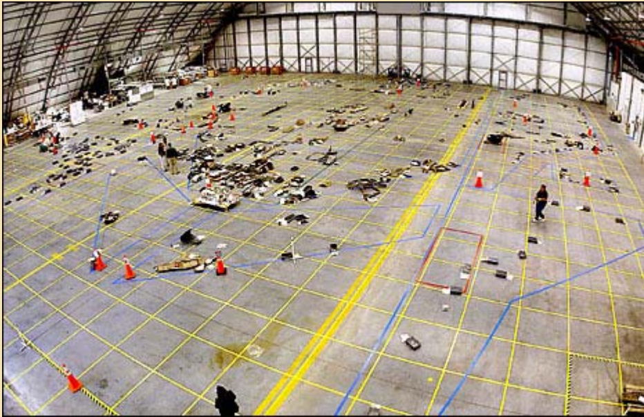
Reassembly of Shuttle at NASA hangar
