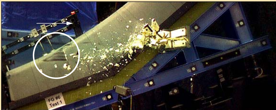
Foam impact testing on wing of shuttle Atlantis
