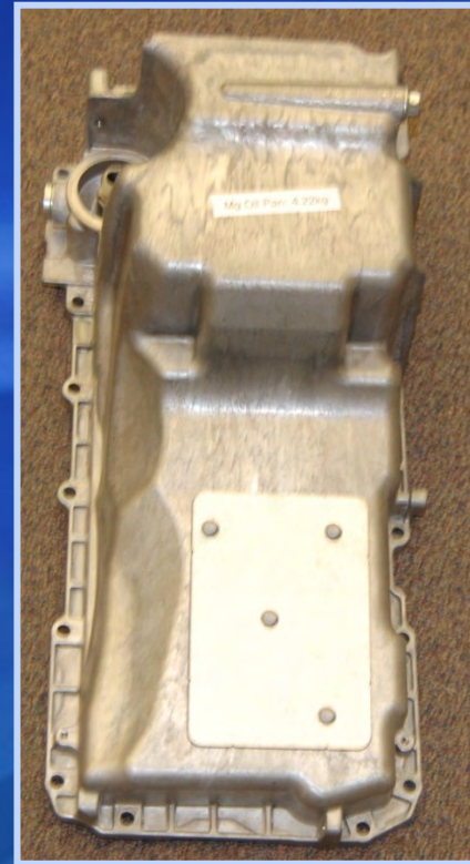
Magnesium (4.2 kg; 30% Reduction) AE44 Alloy
