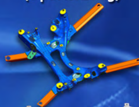
Al Casting-Intensive (6 parts/16 kg)
