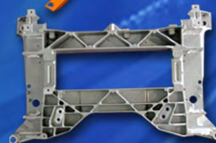
Mg Casting (1 part/10 kg)
