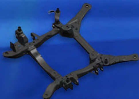
Steel Sheet Construction (46 parts/28 kg)
