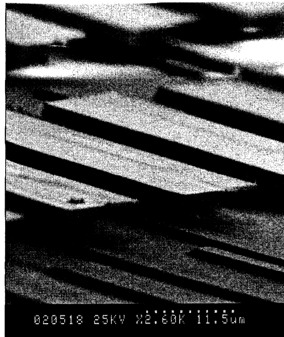
Fig. 1. Array of quantum well modulator diodes bonded to a CMOS chip. The devices are bonded on 62.5 micron x 125 micron centers, for a total of 200 devices on this test chip. (Courtesy Gordon Keeler and Noah Helman, Stanford University)
