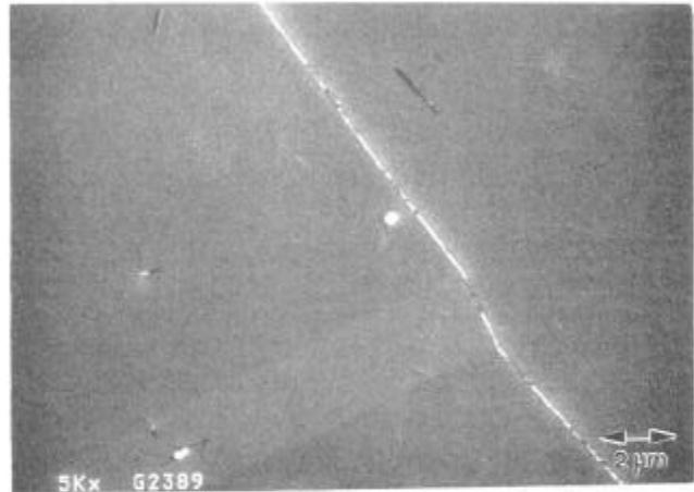
Figure 8. AEREX™ 350 solution treated at 1093°C (2000°F) for 1 hour and aged at 788°C (1450°F) for 4 hours (5000x).
