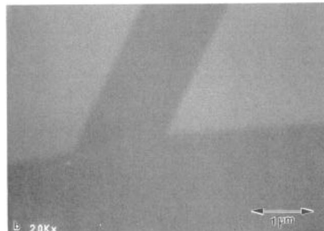
Figure 4. SEM micrograph of AEREX™ 350 solution treated for 1 hour at 1093°C (2000°F). (a) 1,000x and (b) 20,000x
