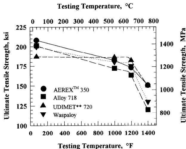
Figure 1. Tensile strength of selected superalloys.
