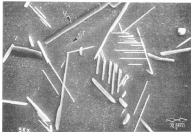
Figure 9. AEREX™ 350 solution treated at 1052°C (1925°F) for 1 hour and aged at 816°C (1500°F) for 4 hours (5000x).
