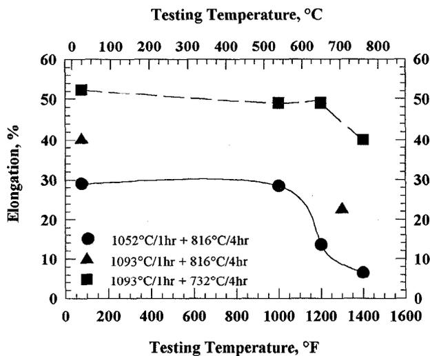
Figure 12. Tensile elongation values for AEREX™ 350.
