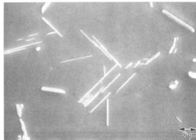
Figure 5. AEREX™ 350 solution treated at 1052°C (1925°F) and aged at 732°C (1350°F) for 4 hours (5000x).
