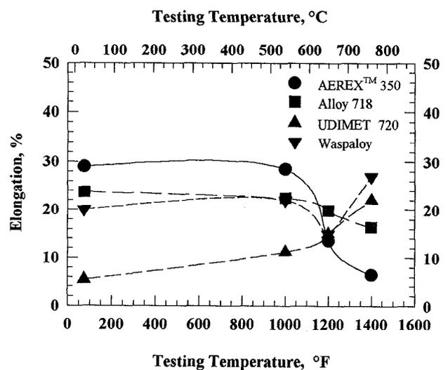
Figure 13. Tensile elongation values for selected superalloys.
