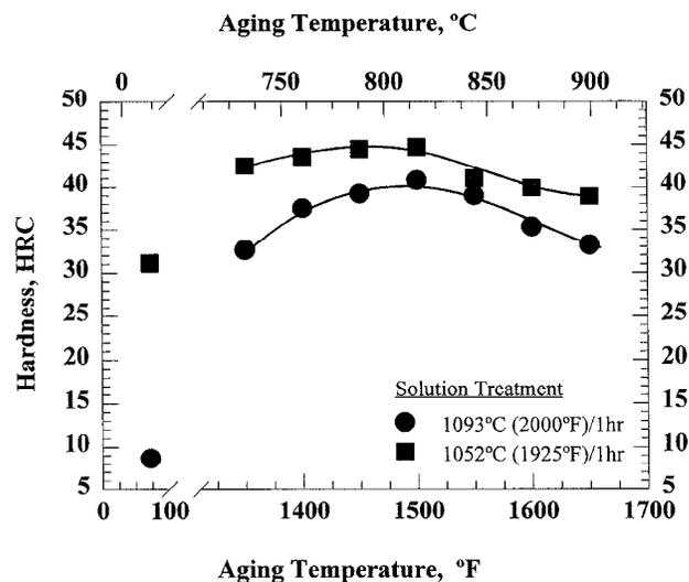
Figure 2. Aging curve for AEREX™ 350.
