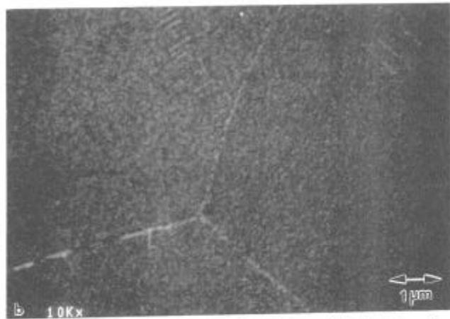
Figure 10. SEM micrograph at (a) 5,000x and (b) 10,000x illustrating AEREX™ 350 solution treated at 1052°C (1925°F) for 1 hour and aged at 899°C (1650°F) for 4 hours + 816°C (1500°F) for 4 hours.
