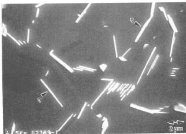
Figure 3. SEM micrograph of AEREX™ 350 solution treated for 1 hour at 1052°C (1925°F) illustrating the presence of eta ( $\eta$ ) phase. (a) 1,000x and (b) 5,000x
