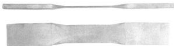
Figure 8: Simulated airfoil test specimen designed to evaluate impact damage at leading edges.
