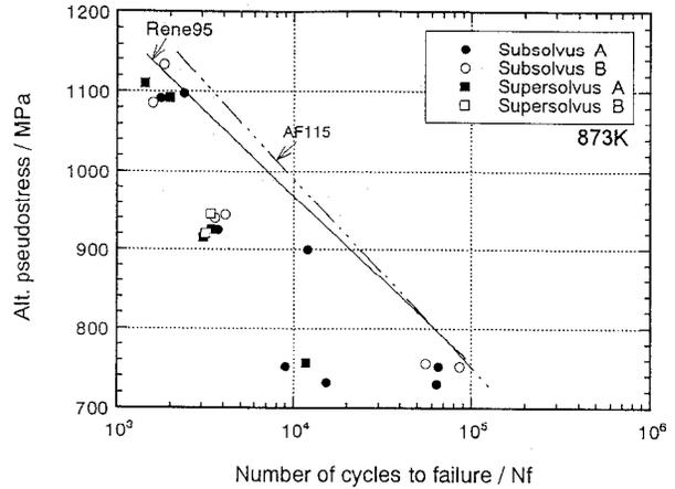
Figure 5 LCF properties comparison between P/M U720 and AF115, Rene95 at 873K.
