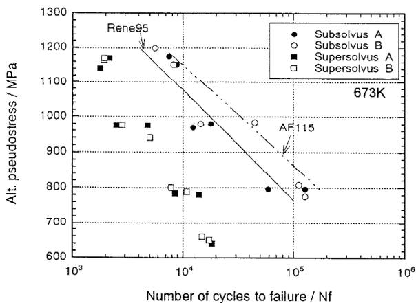
Figure 4 LCF properties comparison between P/M U720 and AF115, Rene95 at 673K.
