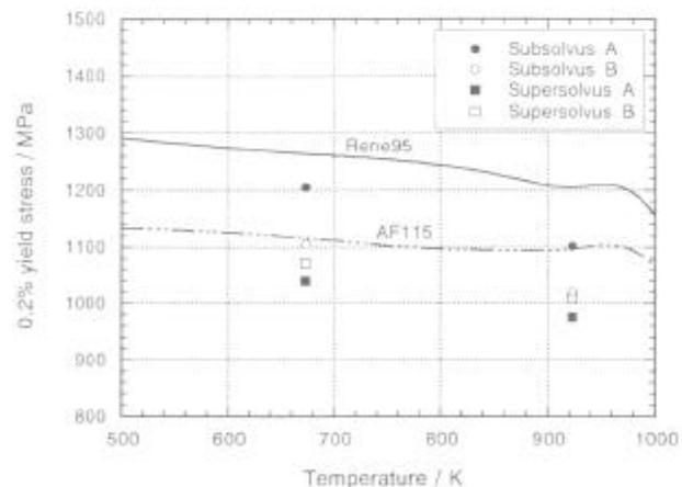
Figure 2 Tensile properties comparison between P/M U720 and AF115, Rene95
