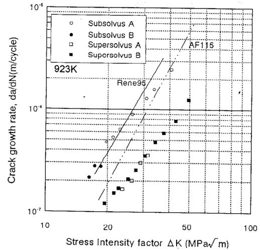
Figure 6 Fatigue crack growth properties comparison between P/M U720 and AF115, Rene95.
