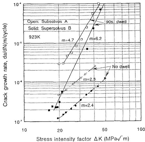
Figure 7 Dwell time effect on fatigue crack growth properties of P/M U720
