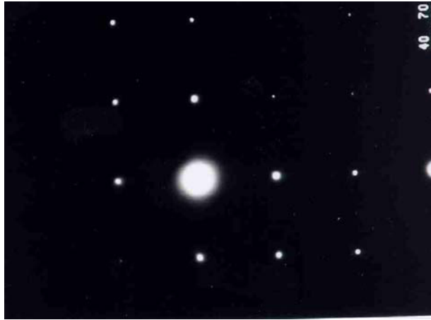
Figure 7. TEM (100)-diffraction pattern of the IN 718 material in the as-welded condition at a distance of 500 \mu\text{m} from the weld seam where \gamma'' precipitates are completely dissolved (no superlattice reflections)
