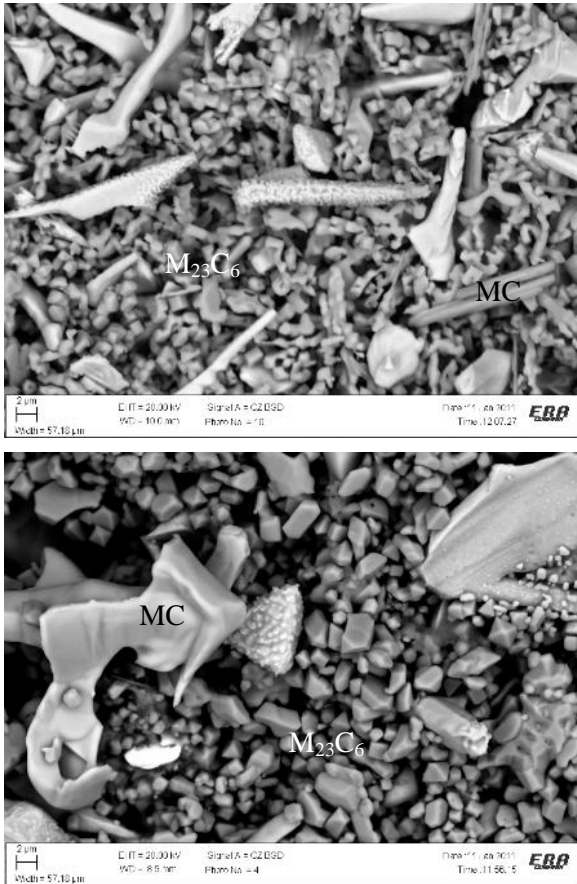
Figure 4: Formation of the M_{23}C_6 after 16,000 hours exposure at 875°C (upper) and 950°C(lower)
