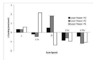
Figure 11. Plot showing ΔCracking (Edgeline Cracking - Midline Cracking values) for complete data sets. The lower energy builds (faster scan speeds) show a clear concentration of the grain-boundary cracking grouped in the middle of the sample.
