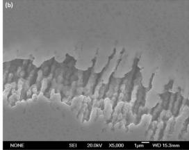
Figure 6. Micrographs showing crack detail in a 'high-energy' build (P2; 1.5v), (a) the dominance of the 'jagged' cracks which show little directionality with respect to the direction of grain growth (build direction). (b) a higher magnification image of a typical 'jagged' crack; note the dendritic growth from either side suggestion the crack has opened during a semi-liquid state typical of a solidification crack.
