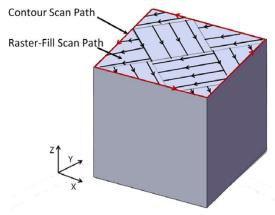
Figure 3. Schematic representation of the laser scanning regime for each layer; The raster filled area is scanned in 5 mm  $\times$  5 mm 'islands', this 'chess-board' pattern moves by 1 mm in both X and Y with each layer. The contour is scanned following the raster fill.
