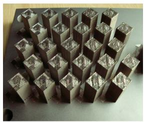
Figure 4. Photograph of matrix of blocks processed with varying scan speeds and laser powers
