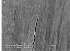
Figure 8. Grain-boundary crack detail: (a) a typical EBSD map of a grain-boundary crack observed in the as-fabricated material. (b) a backscattered SEM micrograph of a similar crack in high magnification; note the fine elongated grains and the particular carbide precipitates along the boundaries including the crack boundary.
