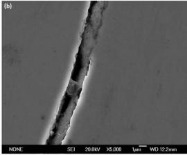
Figure 7. Micrographs showing crack detail in a 'low-energy' build (P1; 2.5v). (a) the dominance of the grain-boundary crack lying dominantly in the build direction. (b) a higher magnification image of a typical grain-boundary crack; note the clean edges indicating that the crack formed in the solid state.
