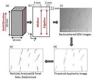
Figure 5. Schematic representation of sampling and analysis method:(a) blocks were sectioned longitudinally (parallel to build direction); (b) 30 images takes along midline and edgeline at 500µm intervals; (c) following standard grinding and polishing, low magnification BSe SEM images reveal cracks; (d) threshold applied to image to isolate cracks; and (e) image analysis carried out to determine feret max. of each crack segment
