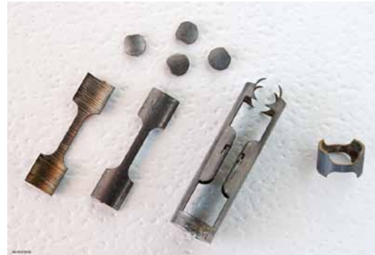
Machined tensile, ring pull, and TEM disk specimens.
