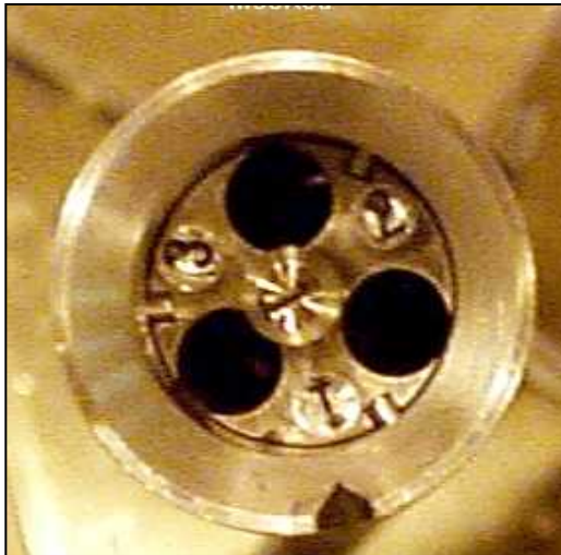
Top view of capsule basket with flux monitor wires inserted
