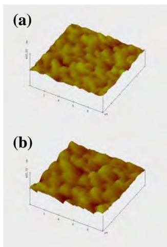
Fig. 4 AFM images showing the surface morphology of 3C-SiC films for (a) sample No. 4 and (b) sample No. 5.
