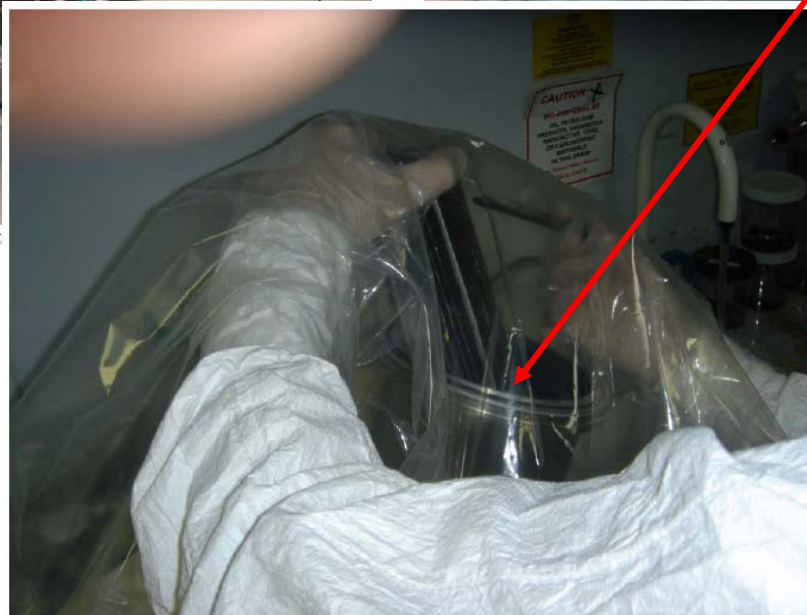
Harvesting nanomaterials inside glove bag, inside down draft hood.
