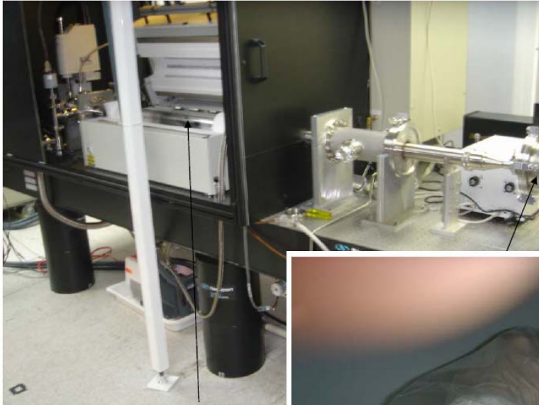
Laser ablation set up. Quartz tube holds laser target and nanomaterials.
