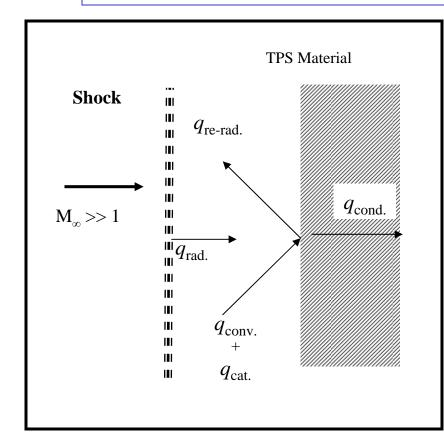
High emissivity coatings increase the reradiated heat-flux and thereby reduce the heatflux to which the material must respond:
