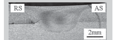
Figure 9. Macrosection of the plate joined using lap welds under optimum FSW condition. 3
