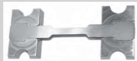
Figure A. A dog-bone shaped sample used for tensile tests.
