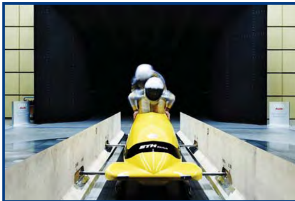
Figure 2. SBSV athletes and the CITIUS endure the wind tunnel test, where the sled was challenged to withstand a 150 kilometer per hour headwind. (Courtesy ETH Zurich)
