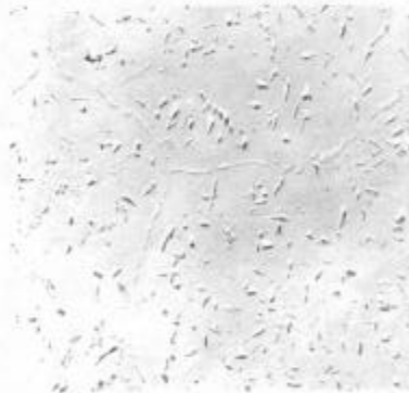
(b) 10M6N solution treated at 1200°C
