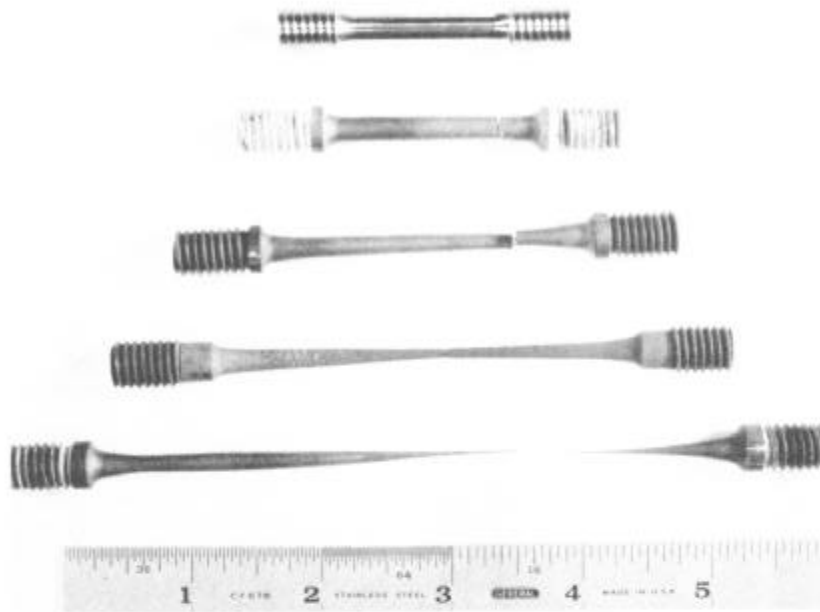
Figure 19. As-Extruded Test Bars Superplastically Deformed at 1900°F at Strain Rates From 0.5 min -1 to 0.01 min -1 . Bar at top is Size of Undeformed Tensile Specimen
