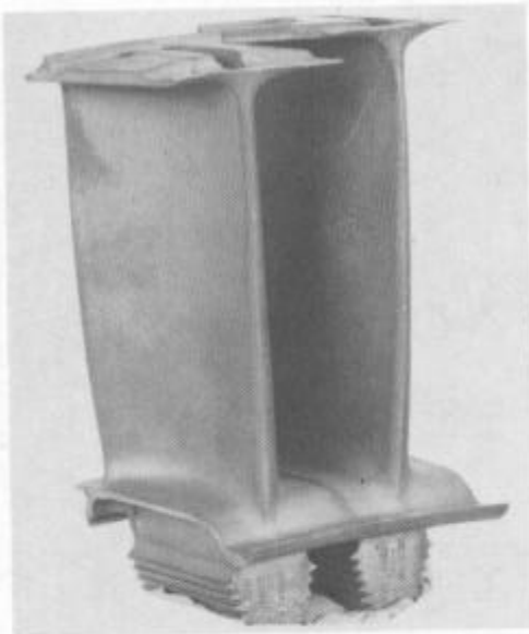
Single Crystal Blade/D.S. Blade Fig 6. D.S. and single crystal blades engine tested at high stator outlet temperature showing difference in creep growth.
