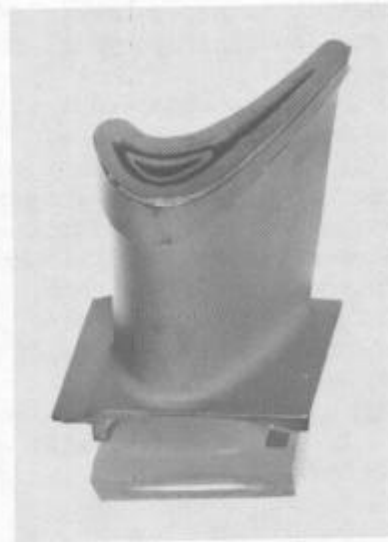
Figure 3. Complex cooled blade used as castability testpiece for single crystal alloys.
