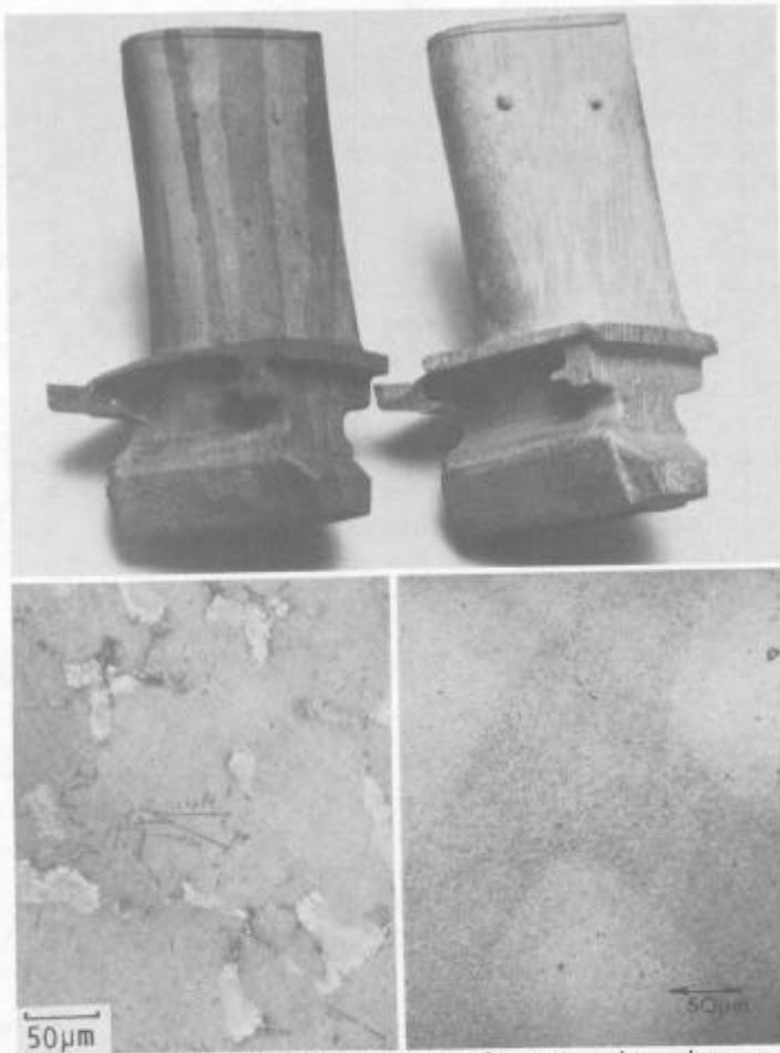
Figure 1. Microstructures and macrostructures of fully heat treated D.S. and single crystal turbine blades.
