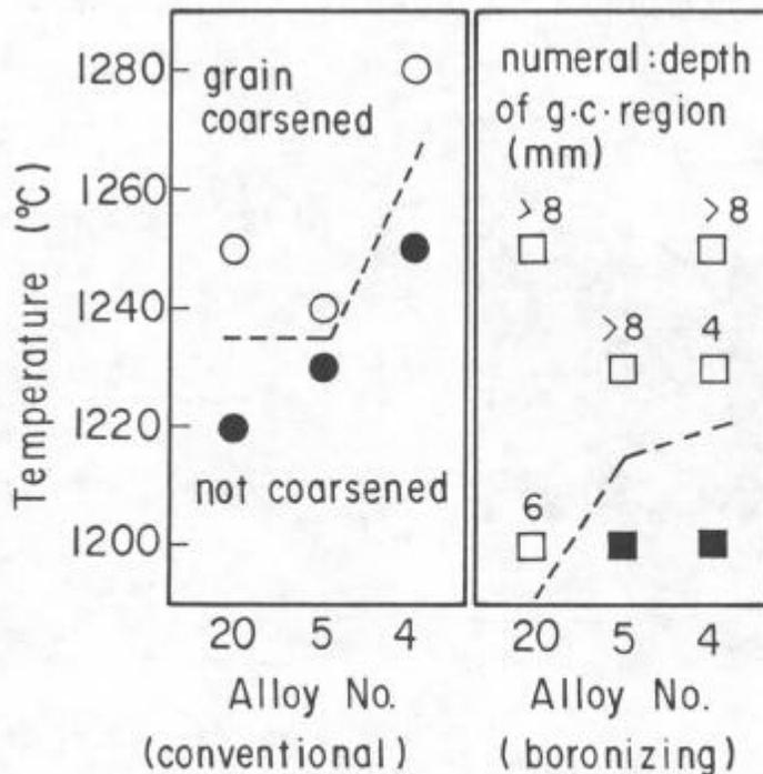
Figure 5 Effect of boronizing on abnormal grain growth temperature
