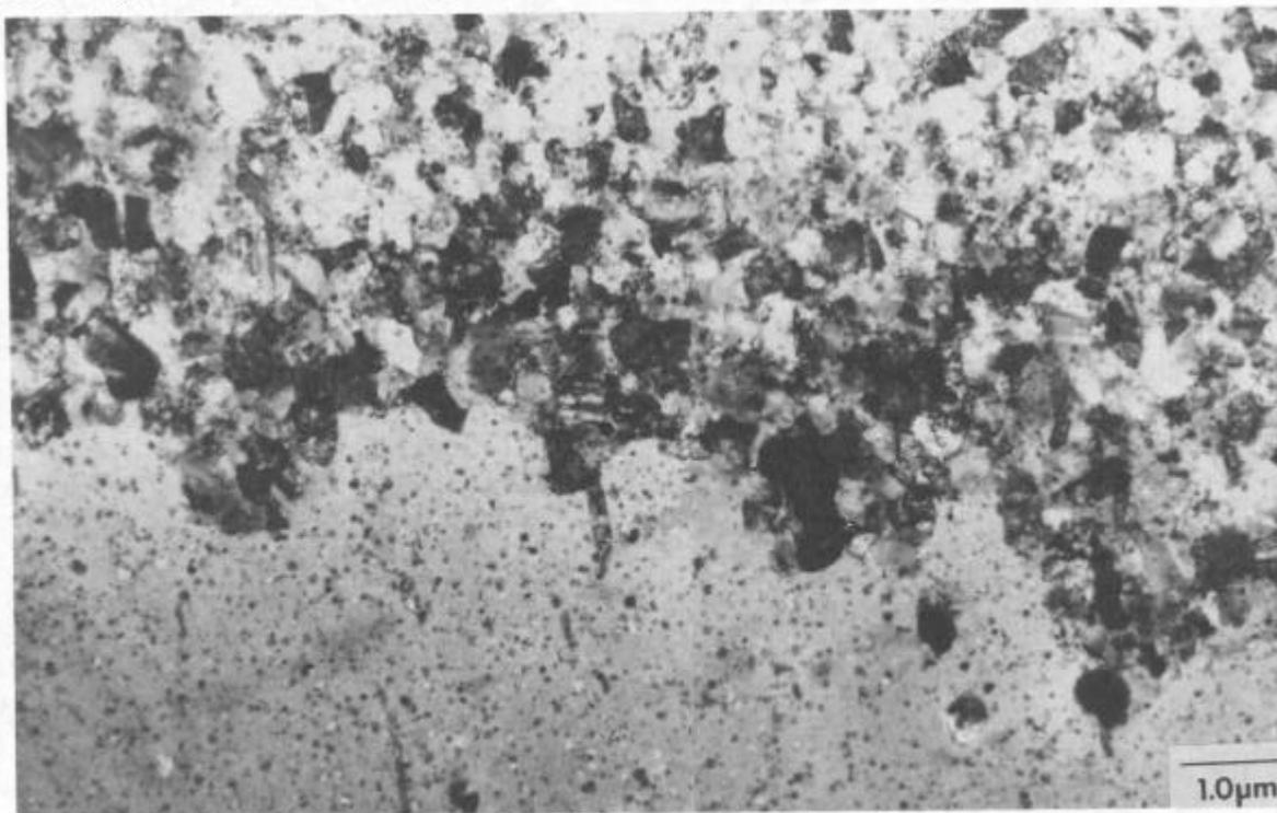
Figure 3 TEM microstructure of coarsely elongated grain and fine grain interface in the zone annealed TMO-2
