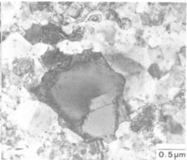
Figure 9  $\gamma'$  grain observed in the as-extruded MA6000
