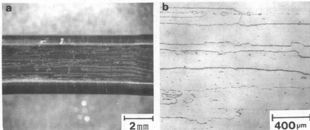
Figure 6 Longitudinal structure of MA6000
