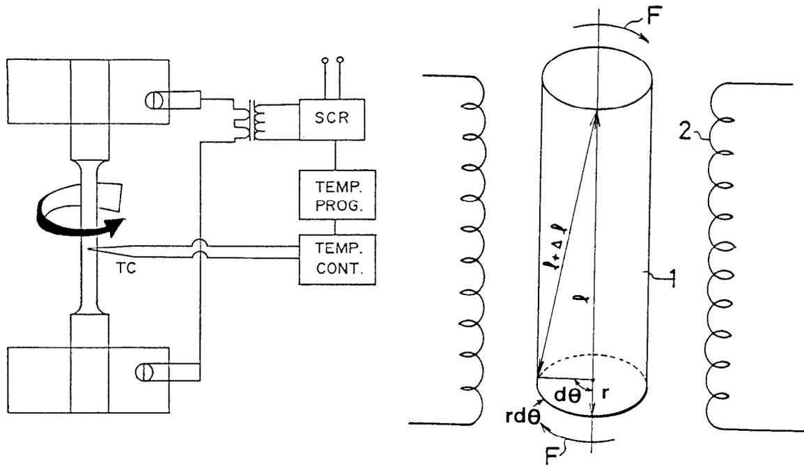
Figure 1 a) Set-up used for high temperature torsional straining
