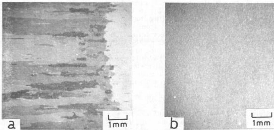
Figure 4 Longitudinal structure of Alloy 20 at 1200°C for 15h,
