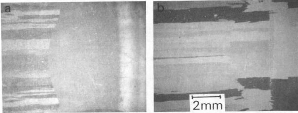
Figure 2 a) Longitudinal macrostructure of TMO-2 as zone annealed, and b) subsequently heated isothermally at 1290°C for 10 min
