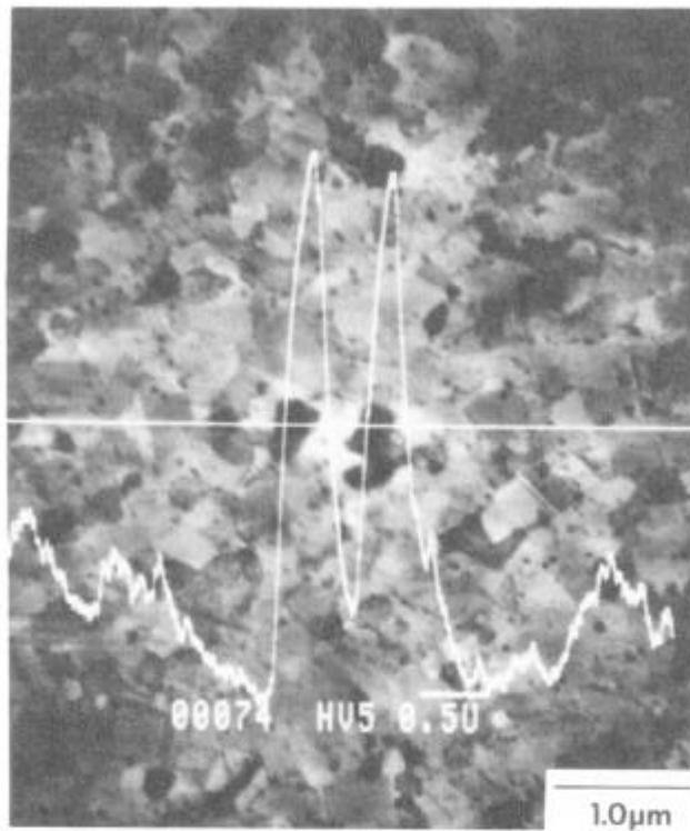
Figure 10 High Cr content grains in the as-extruded MA6000 (Cr line)
