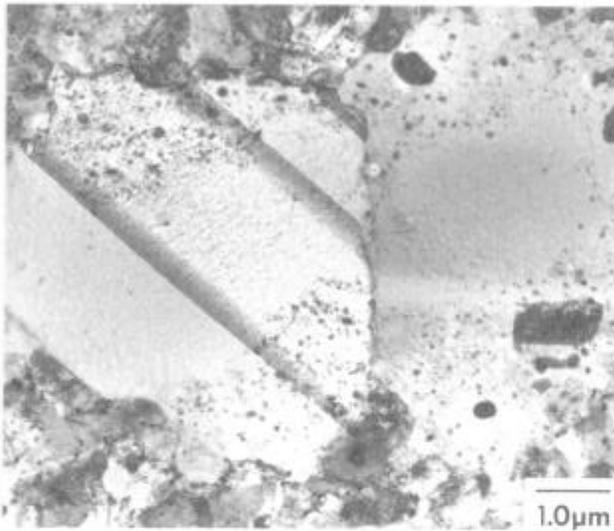
Figure 8 Recrystallized grains observed in MA6000 strain (16%) annealed at 1180°C, (TP11)
