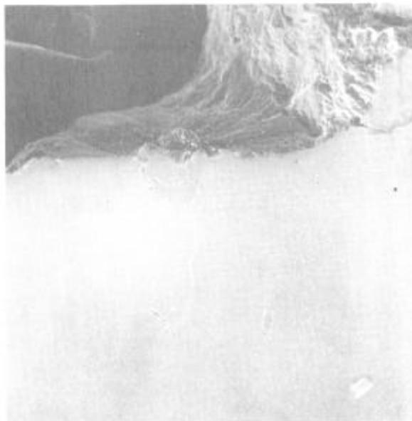
Figure 7: A section taken through a crack initiation site of a sample tested under 'slow-fast' conditions. A crack has initiated on the transverse boundary of a fine, included grain. The outlines of several small grains have been made visible by etching the polished axial section.
