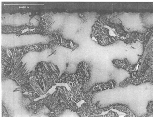
Figure 2: Microstructure of RS5 in the as-cast condition.
