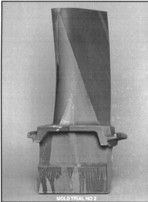
Figure 10: Casting defects in a large single crystal UGT blade
