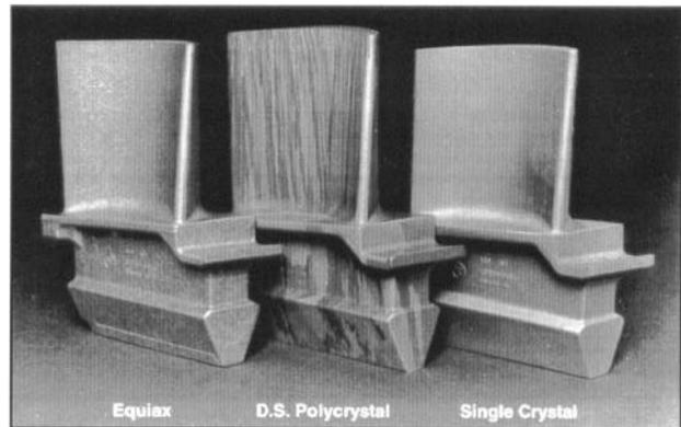
Figure 9: Evolution of grain structures in UGT blades
