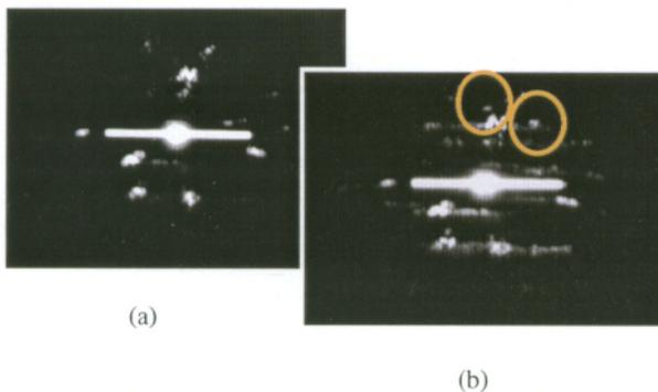
Figure 22: Through transmission SC image (a) no defect (b) internal misoriented grain
