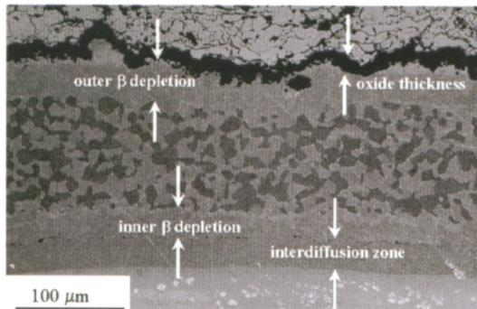
Figure 16: Typical MCrAlY coating after thermal exposure
