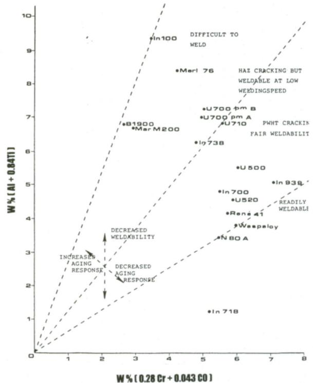
Figure 23: Weldability diagram for a number of nickel-base superalloys and related materials<sup>(31)</sup>
