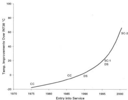
Figure 8: Increase in temperature capability of superalloys in UGTs
