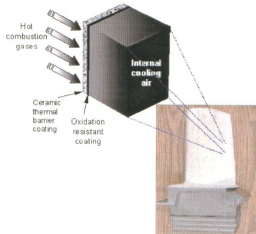
The thermal barrier coating system consists of a metallic bond coat and a ceramic thermal barrier coating (Figure 17). The bond coat provides oxidation and corrosion resistance by forming a slow growing adherent protective aluminum oxide scale, whereas the ceramic top layer reduces the substrate alloy temperature.
