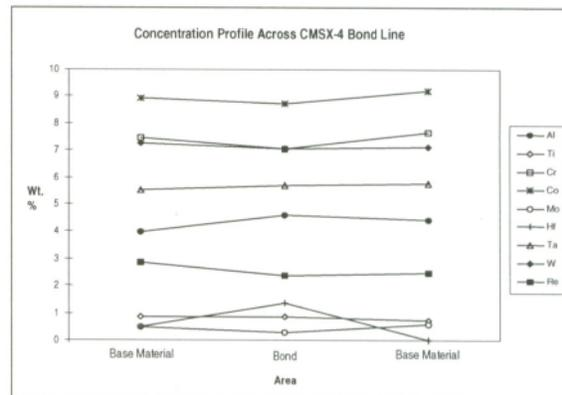
Figure 14: Microprobe analysis across the transient liquid phase bonded CMSX-4 single crystal bond region
