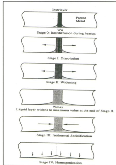
Figure 13: Principle of transient liquid phase bonding<sup>(13)</sup>
