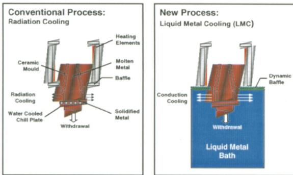
Figure 12: Conventional and liquid metal cooling processes<sup>(8)</sup>
