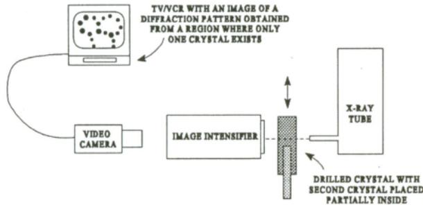
Figure 21: Schematic of SC through-transmission imaging
