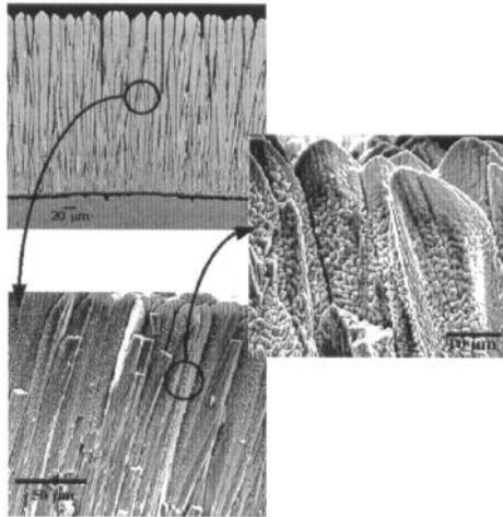
Figure 19: EB-PVD thermal barrier coating
