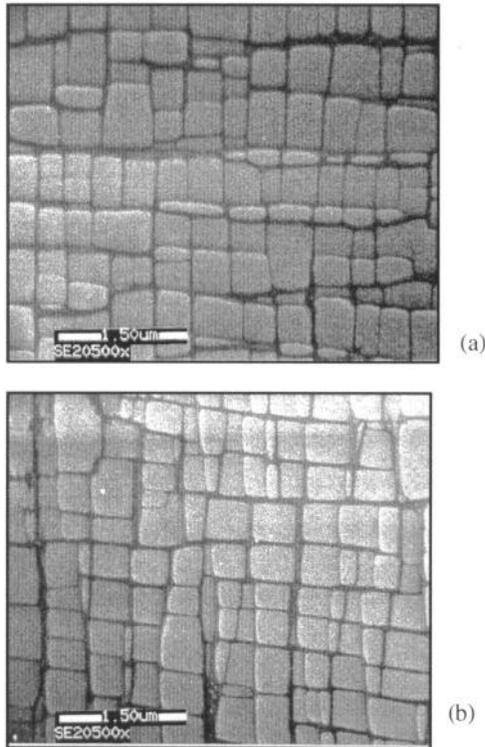
Figure 15: Gamma-prime morphology of a) bond zone and b) base material in bonded CMSX-4 single crystal
