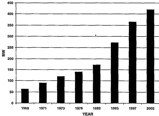
Figure 4: Evolution of UGT plant size
