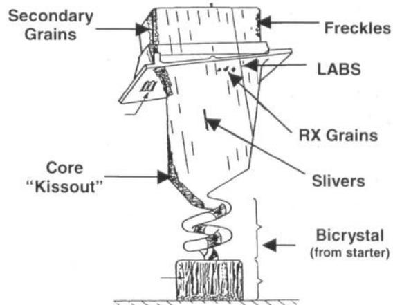
Figure 11: Typical defects in single crystal castings
