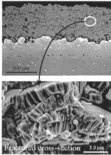
Figure 18: Air plasma sprayed thermal barrier coating
