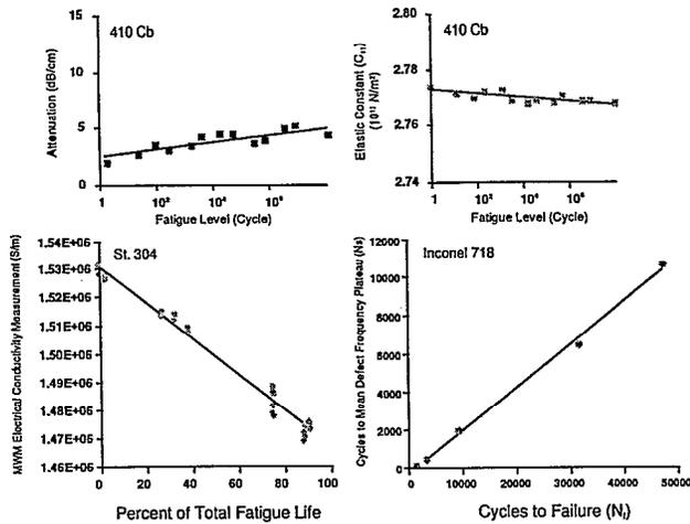
Figure 20: Fatigue damage detection by various NDE techniques<sup>(22-24)</sup>
