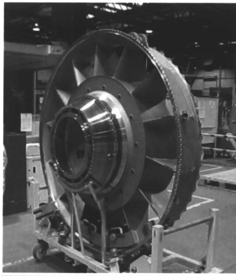
Figure 4. Weldability of Alloy 718 enables application of complex cast structures represented by the GE90 Turbine Rear Frame (matte gray structure with inner and outer annulus connected by integrally cast struts).
