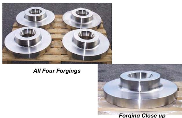
**Figure 5.** View of the René 104 forgings for DHT after ultrasonic inspection and machined to the final DHT shape.
