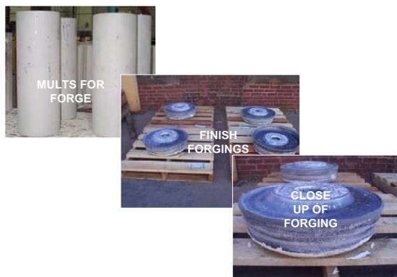
**Figure 4.** View of mults prior to forging, the four completed forgings and a close up of a typical forging.
