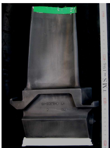
Figure 11. TMS-196 casting trial to a hollow single crystal turbine blade for a land-based gas turbine.
