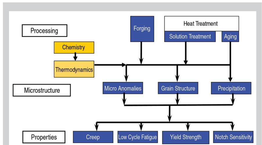
Figure 1. An example of key processing-structure-property linkages for forged nickel-based superalloys.
