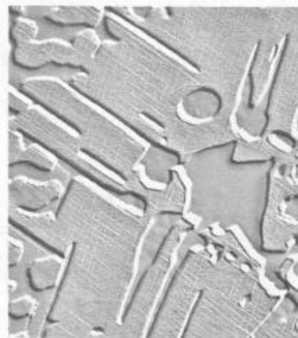
B) Electron micrograph showing acicular MC at 1800°F/5000 hrs. X6000.
