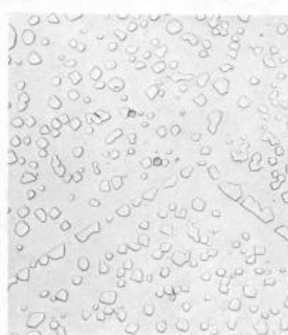
F) Light micrograph showing gamma-prime and M_{23}C_6 in grain boundaries at 1800°F/5000 hrs. X500.
