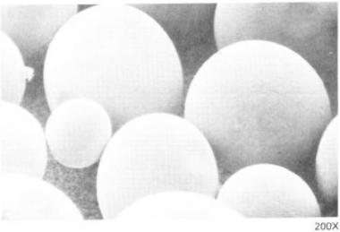
Rotating Electrode process (-60 mesh)
