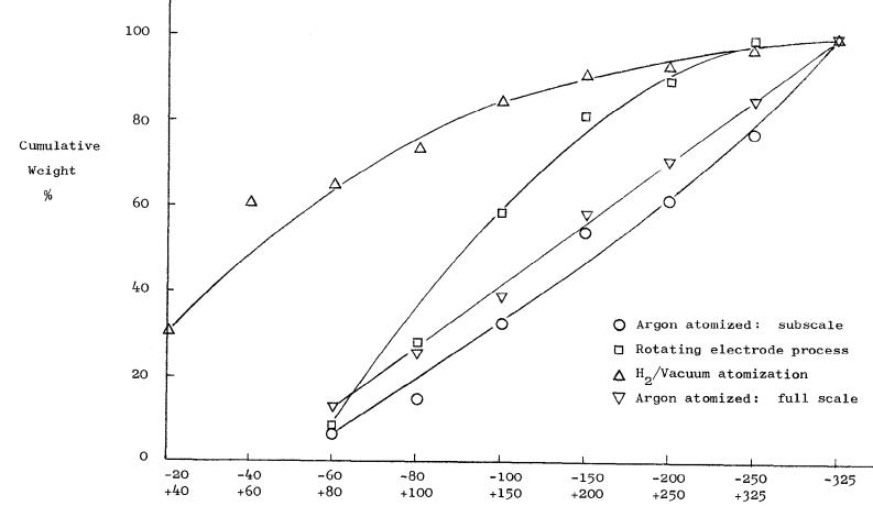
Figure 1: Particle size distribution for three subscale powder lots and average of full-scale pow
