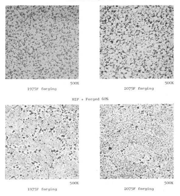
Figure 6: Effect of Forging Temperature on HIP Compacts and Extrusions using Argon Atomized Powders.
