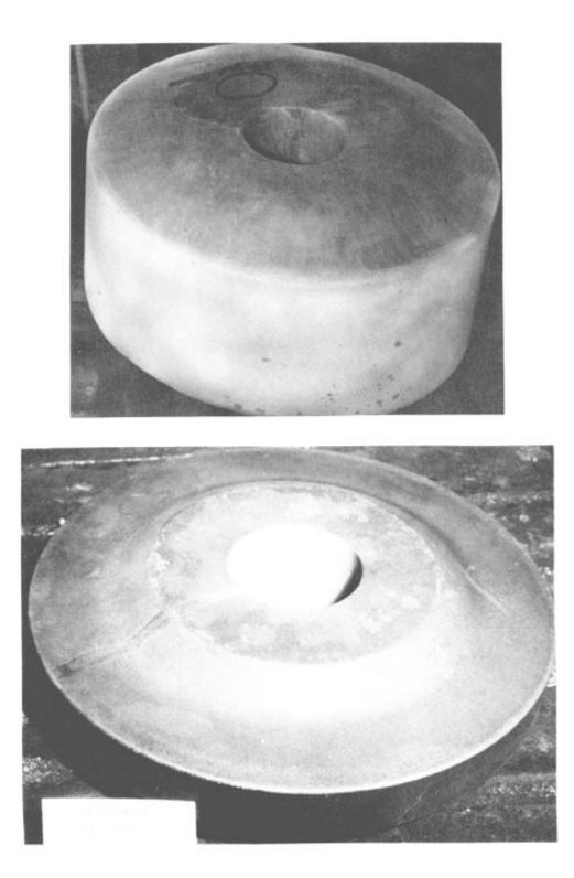
Figure 4: Rene' 95 Full-Scale Forging Preform and Jet Engine Disk Forging. Top: Forging Preform: (15-1/2" OD X 8-1/2" thick) Bottom: Finish Forged Disk: (20" OD X 4" thick at bore)
