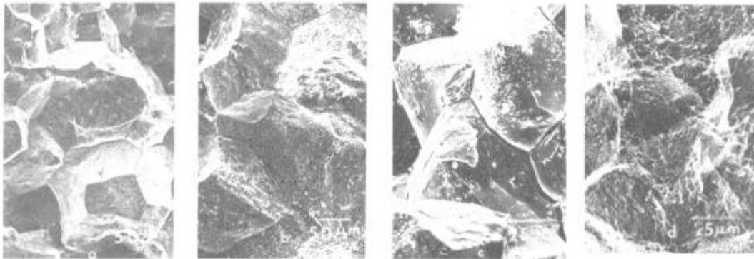
Fig.13 The influence of Mg on fracture mode of GH220 and GH169 alloys
