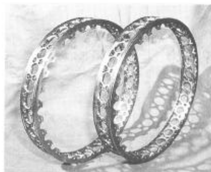
Figure 10 - Alpha-2 GE29 high pressure turbine support ring fabricated from alpha-2(left) and René 41(right).
