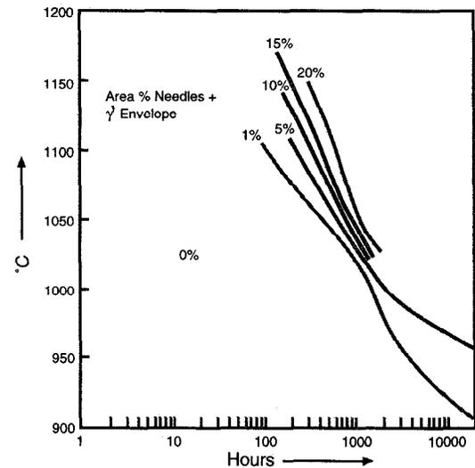
Figure 2: CMSX-10 alloy tendency for TCP phase formation.
