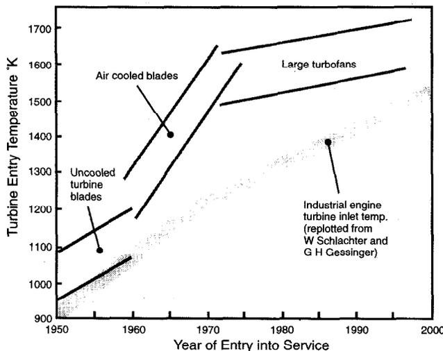
Figure 1: Comparison of civil aero engine take off temperatures and industrial engine turbine inlet temperatures (3).
