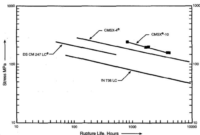
Figure 10: 982°C stress-rupture strength of several alloys.
