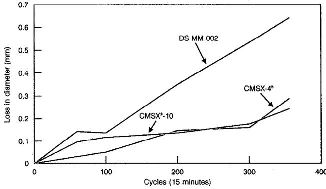
b 1100°C burner rig oxidation
