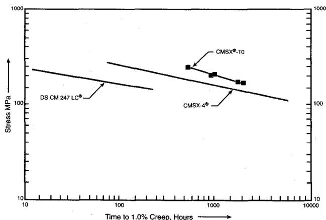
Figure 11: 982°C 1% creep strength of several alloys.
