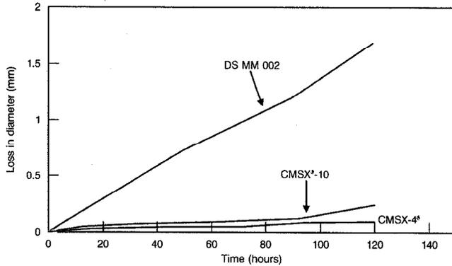
c 950°C burner rig hot corrosion
