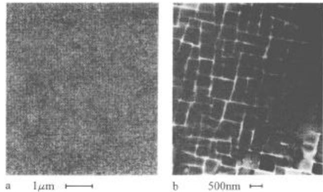
Figure 4: Two views of fully heat-treated CMSX-10 alloy.
