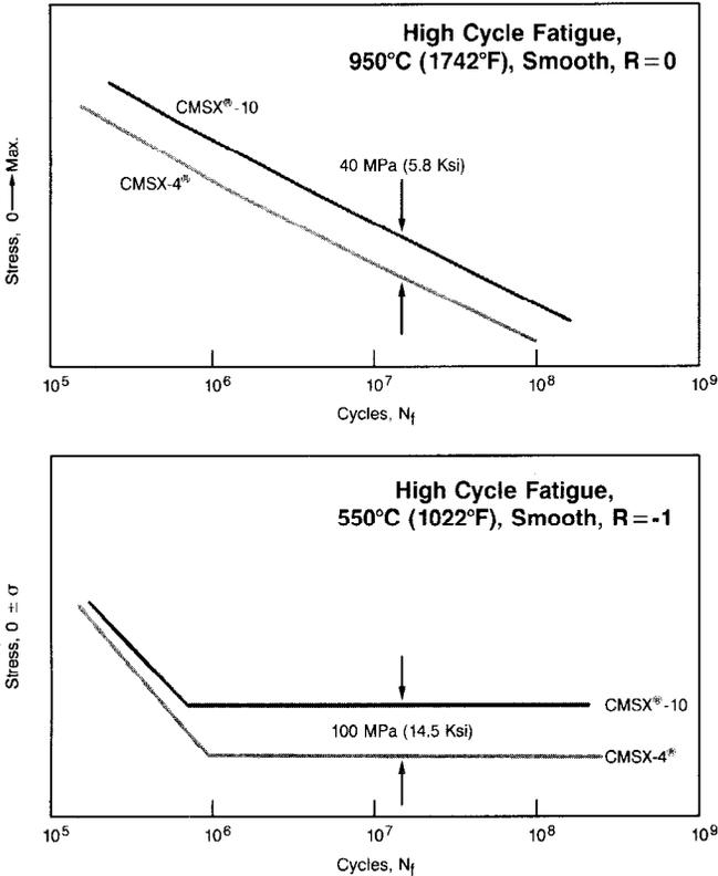
Figure 13: High cycle fatigue behavior of CMSX-10 and CMSX-4 at 550°C and 950°C.
