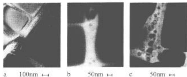
Figure 5: The CMSX-10 alloy aged at (a) 1,152 °C, (b) 1,152 °C + 871 °C and (c) 1,152 °C + 871 °C + 760 °C.
