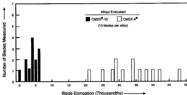
Figure 8: Post turbine engine test blade growth measurement results.
