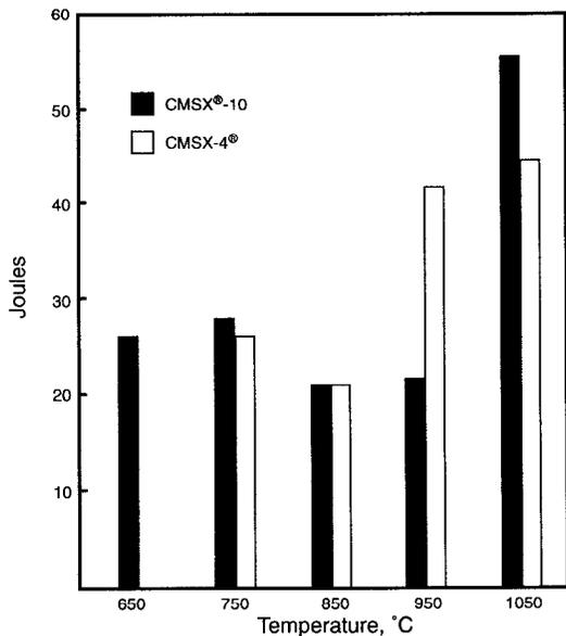
Figure 7: CMSX-10 impact strength. Cylindrical specimen, 7.2 mm diameter x 55 mm long.
