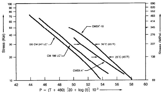
Figure 9: 1.0% Larson-Miller creep strength of several alloys.
