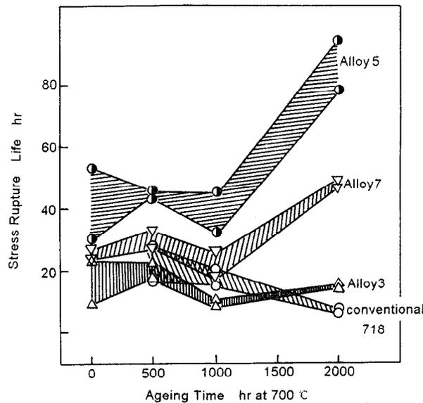
Fig.3 Variation of Stress Rupture Life with Ageing Time for Modified and Conventional 718 Alloys
