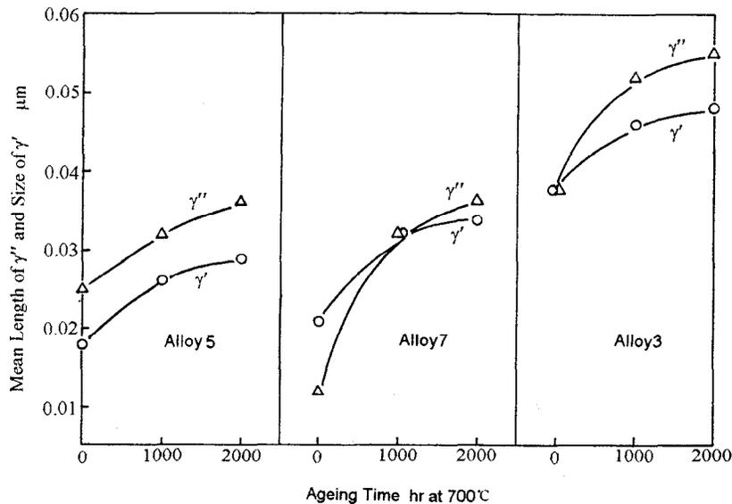
Fig.5 Variation of Mean Length of  $\gamma''$  and Size of  $\gamma'$  with Ageing Time at  $700^\circ\text{C}$  for Alloy 5, Alloy 7 and Alloy 3
