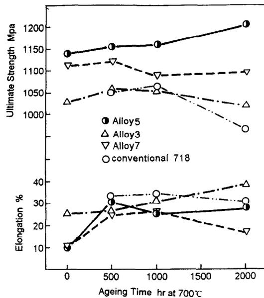
Fig.2 Variation of Ultimate Strength and Elongation at 700 °C with Ageing Time for Modified and Conventional 718 Alloys
