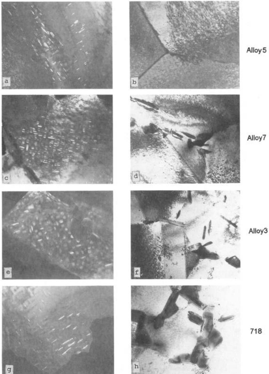
**Fig.4** TEM dark and bright field images of Alloys Aged for 2000hr at 700 °C
