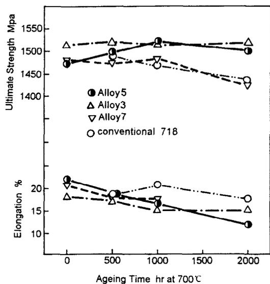
Fig.1 Variation of Ultimate Strength and Elongation at 25 °C with Ageing Time for Modified and Conventional 718 Alloys
