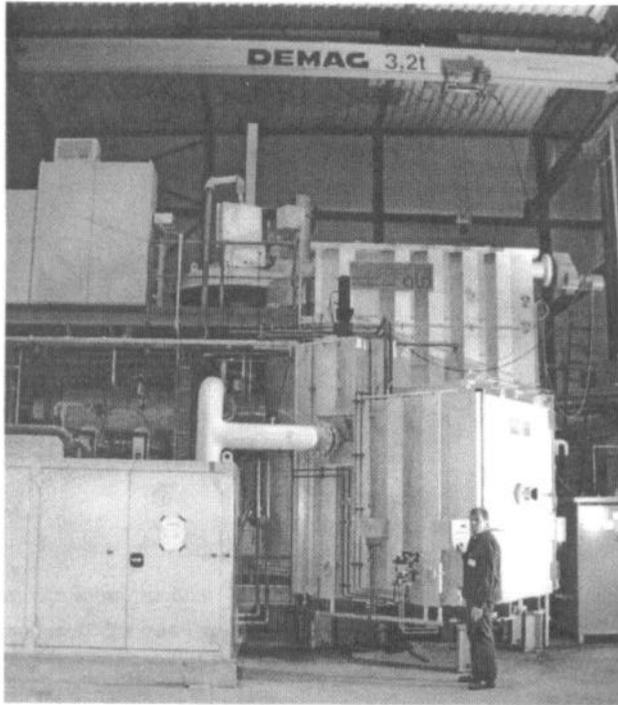
**Figure 1:** Industrial scale LMC-furnace at DONCASTERS Precision Castings - Bochum GmbH, Germany. This furnace is in operation since mid of 1999.
