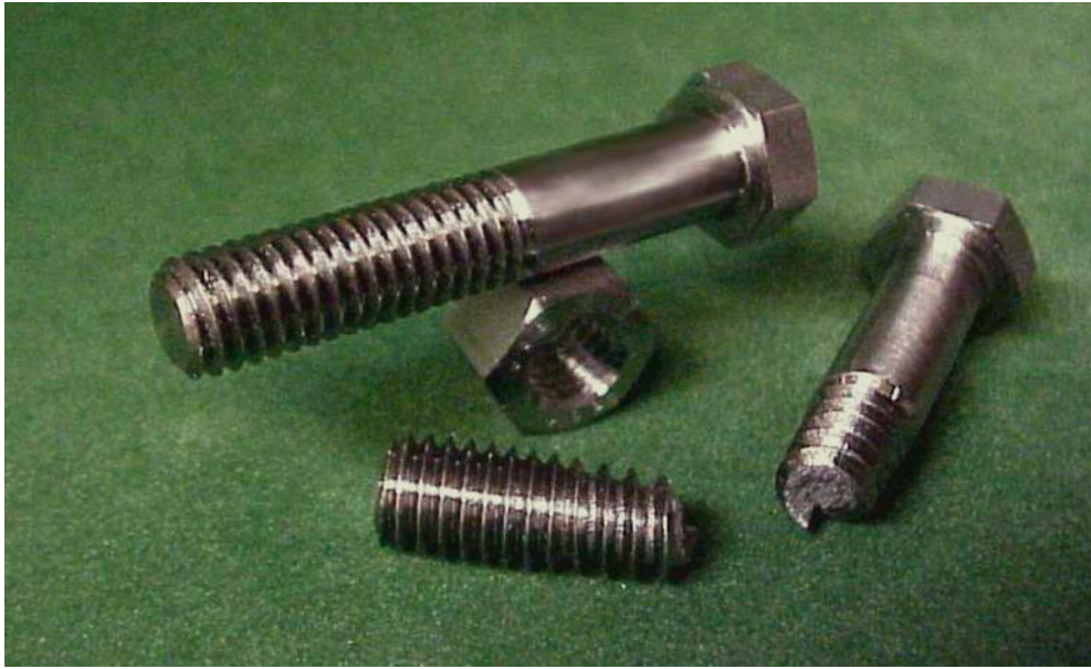
Figure 8 – Fasteners fabricated from high strength, corrosion-resistant materials such as alloys 625 and 725 are widely used in marine service. Their toughness is evident by the ductile fracture of the test bolt.
