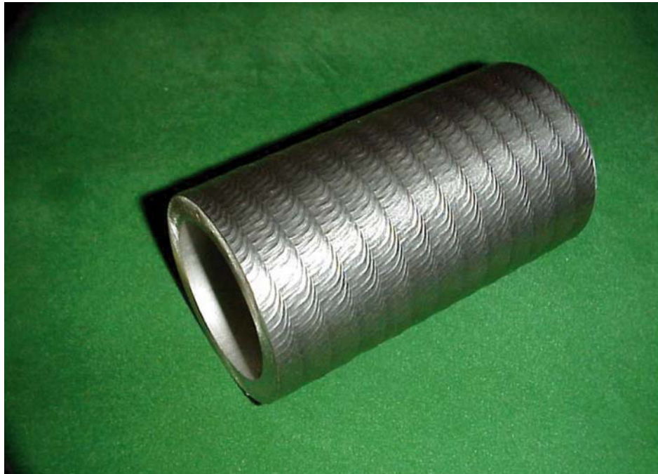
Figure 7 – Alloy Steel Boiler Tube Weld Overlaid with alloy 625
