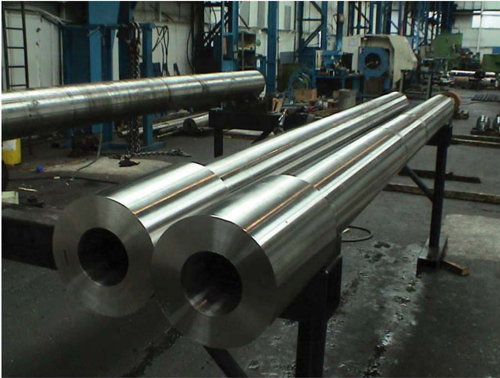
Figure 10 –Downhole hanger for an oil well machined from alloy 725 bar. This component must support the weight of the entire well casing. Requirements of service are high strength and resistance to general and localized corrosion under sour (acid halide + H 2 S) well conditions.
