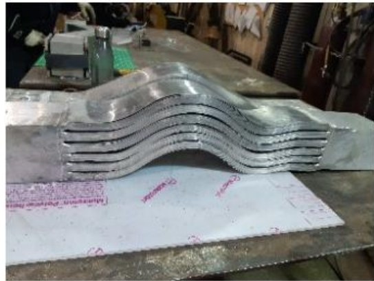
Final compression cycle | unloaded deformed shape immediately after u_L = 220 mm (COMP-3)
