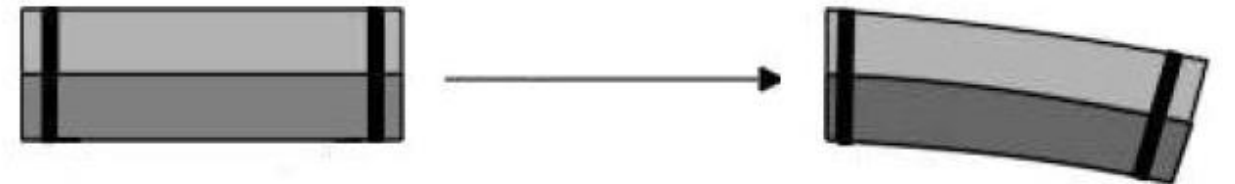
Differential thermal expansion generates bending stresses
