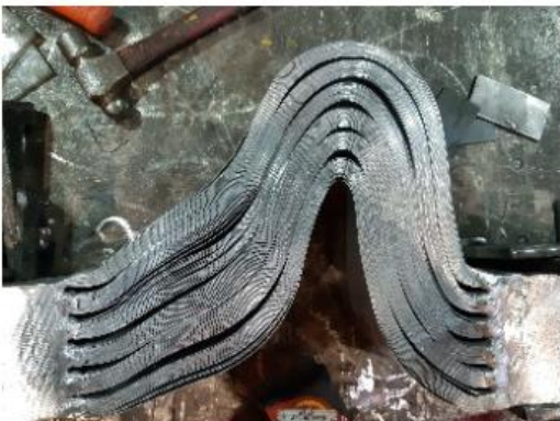
Final compression cycle | unloaded deformed shape immediately after u_L = 220 mm (COMP-3)
