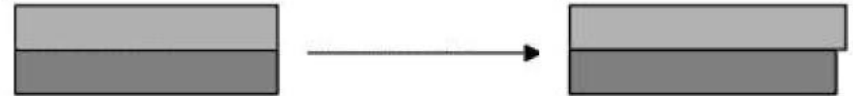
Differential thermal expansion generates bending stresses
