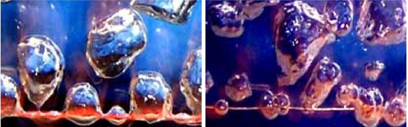
Fig. 4. Top Photo: De-ionized water at 1 MW/m<sup>2</sup> heat flux (observe the vapor film coating the heated wire). Bottom photo: Nano fluid at 1 MW/m<sup>2</sup> heat flux (fluid is still wetting the surface). (from Kim, S. J., 2007)
