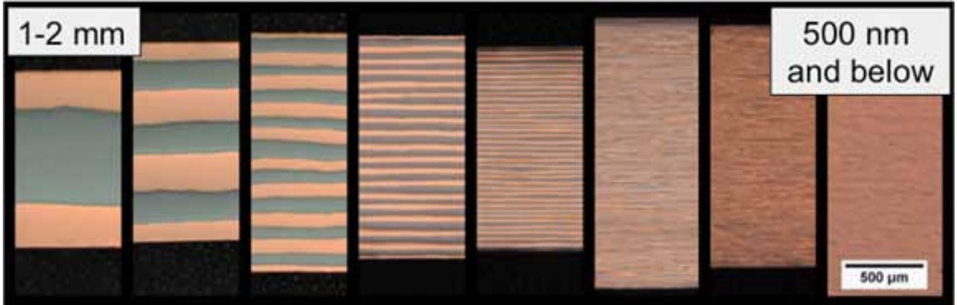
Fig. 10. Optical micrographs of Bulk Cu-Nb multilayers produced via Accumulative Roll Bonding. Starting layer thicknesses are on the order of millimeters, and the layer thicknesses can be refined down to 10 nanometers while retaining bulk sample dimensions and a continuous layered structure.
