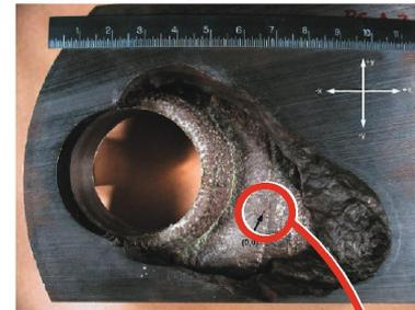
(e) LPSCC crack in cladding
