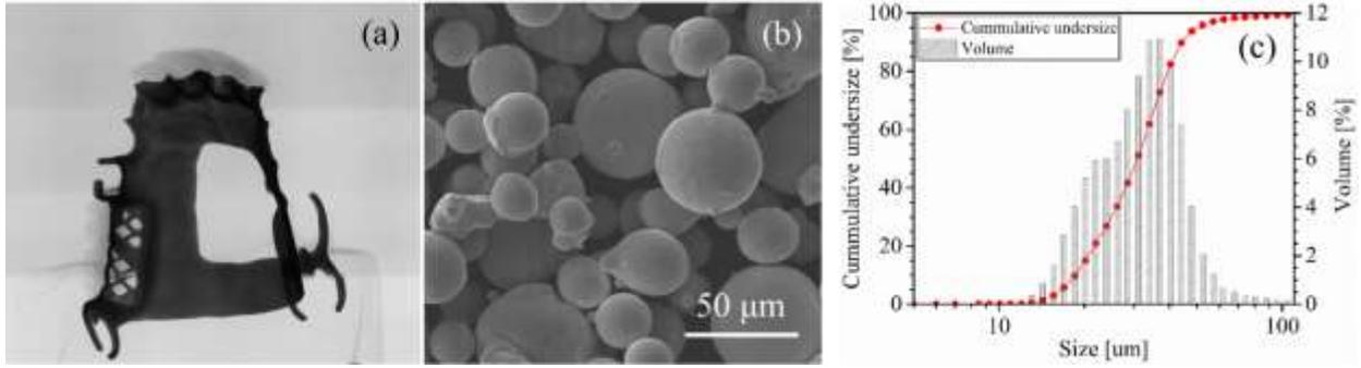
Figure 1. (a) The scanned 3D model obtained from the denture framework using  $\mu$ CT, (b,c) SEM and particle size distribution of the used powder for printing.
