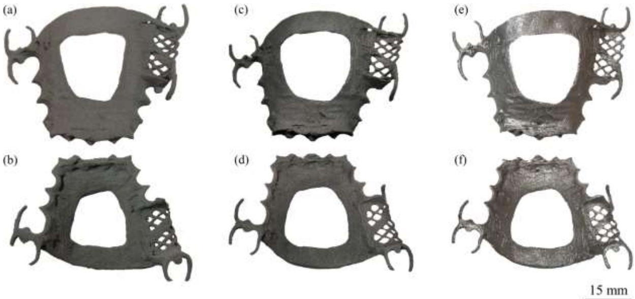
Figure 2. Top and bottom view of the (a,b) printed, (c,d) sintered, and (e,f) polished denture.
