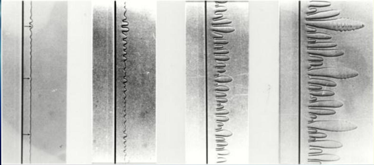
Development of cells to deep cells to dendrites with time during the directional solidification of a transparent alloy in thin samples that give two-dimensional pattern evolution under diffusive growth conditions. -- *succinonitrile-camphor*, Courtesy of Rohit K. Trivedi, Iowa State University
