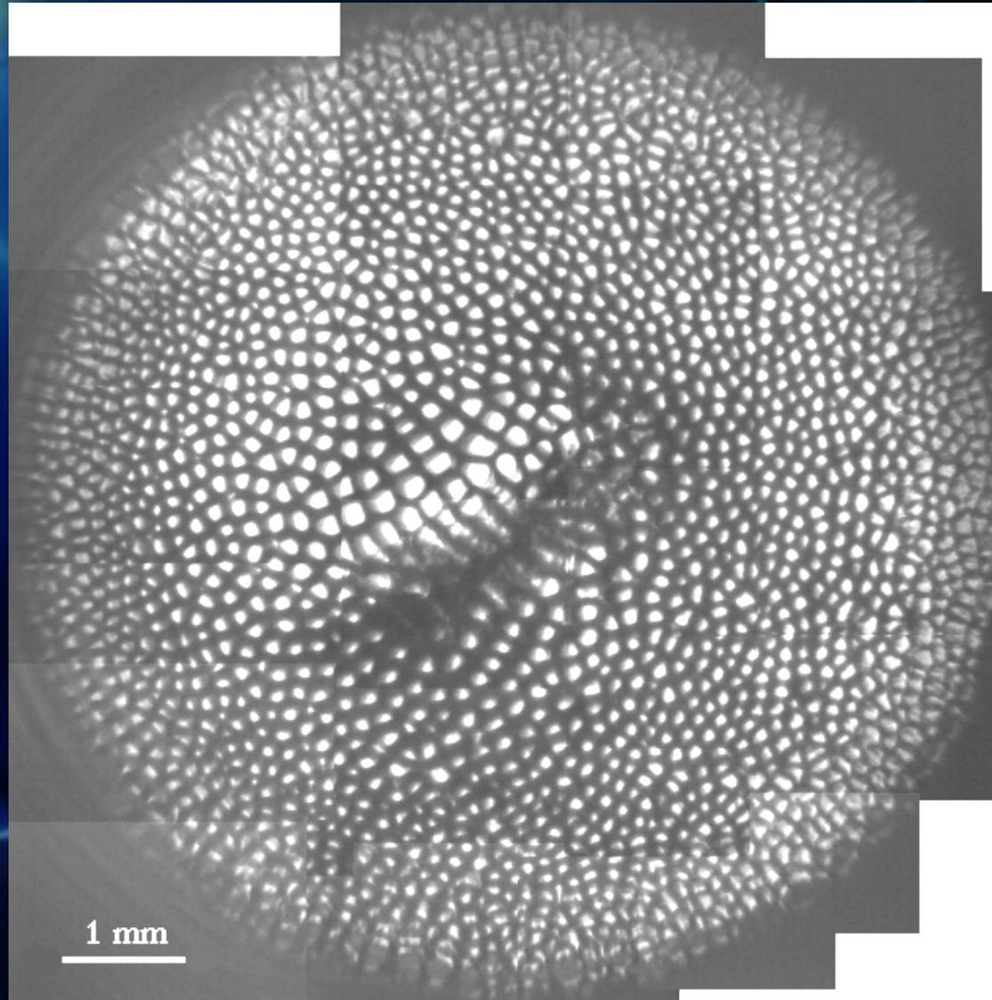
**Interface pattern evolution in three-dimension, observed in bulk samples that shows a very inhomogeneous pattern evolution due to the presence of fluid flow—convection on Earth disrupts the pattern and uniformity -- succinonitrile-camphor, Courtesy of Rohit K. Trivedi, Iowa State University**
