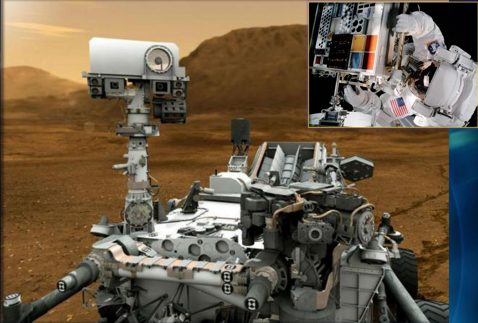
**A coating that survived long-term exposure on the ISS as part of the MISSE investigation is now protecting the Mars Curiosity Rover's critical power unit from static electricity as it collects data on Mars.**
