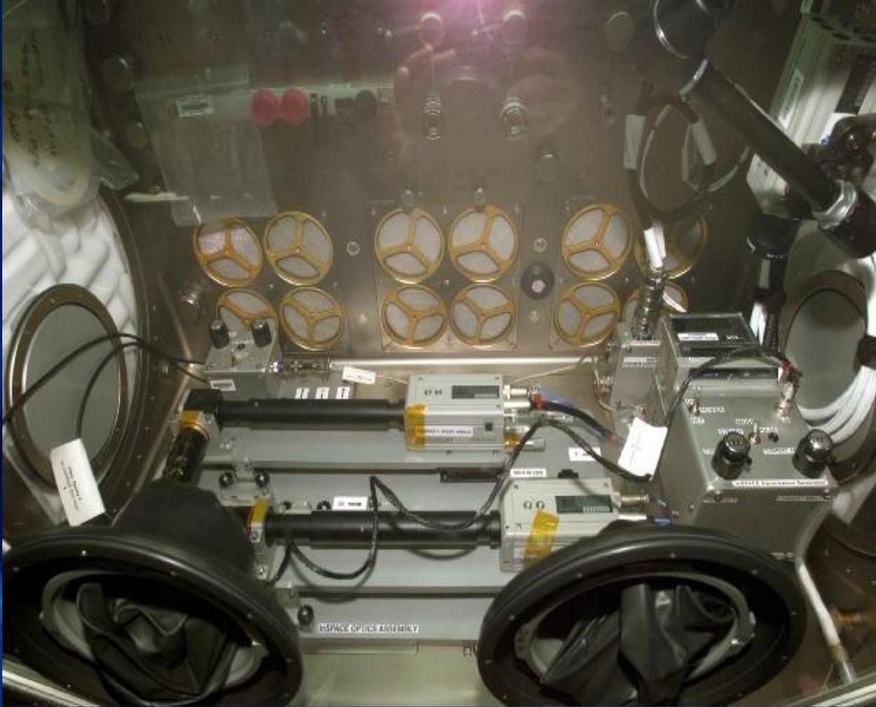
**Smart Materials** – Studies on the *International Space Station* have investigated the internal structure of fluids that change properties in response to magnetic fields, without additional gravitational effects. Resulting technology has promise to improve the design of structures, such as buildings and bridges, to better withstand earthquakes.
