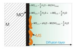
General corrosion manifests through combined effects of water chemistry and surface reactivity. OLI has combined these fundamental electrochemical mechanisms to enable corrosion prediction on carbon steel, <u>Corrosion Resistant Alloys</u>, or CRAs (nickel-base alloys and stainless steels), Cu, and Cu-Ni alloys. The impact of acids, bases, salts, acid gases, temperature, pressure, shear, and film formation are also quantified.
