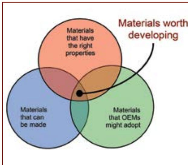
curtailing the need to synthesize and test a large palette of contenders, as illustrated as a Venn diagram in Figure 1. The process of down-selection—the systematic rejection of unacceptable solutions—is achieved by applying filters to the pool of candidates. The sooner we make a No-Go decision, the more the resources that can be applied to the remaining candidates and the early application of available filters accelerates the process.
