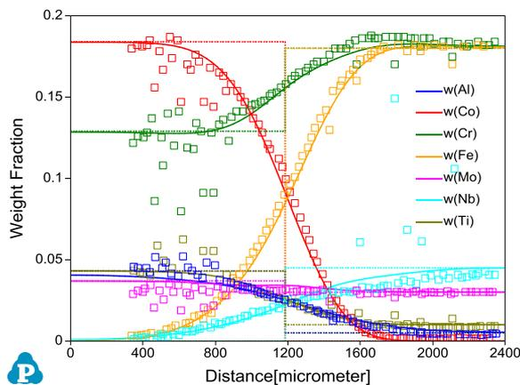
Figure 1: Diffusion between IN100 and Alloy 718 at 1150°C for 1000 hours, experimental data are from Campbell et al., Materials Science and Engineering, A 407 (2005), 135-146.
