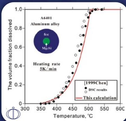
Dissolution of Mg<sub>2</sub>Si precipitate in Alloy A6401
