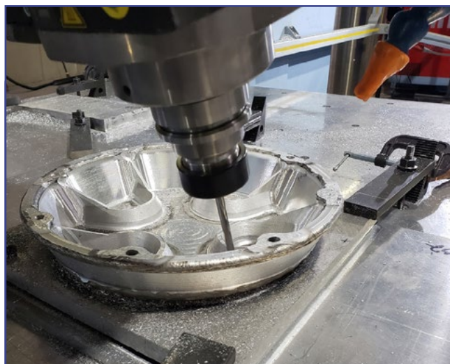
Early stages of manufacturing a cryogenic tank with integral cooling passages.
