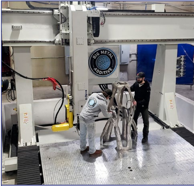
Parts 8 ft tall can be produced on this large BMA machine with a work table 12 ft x 12 ft.
