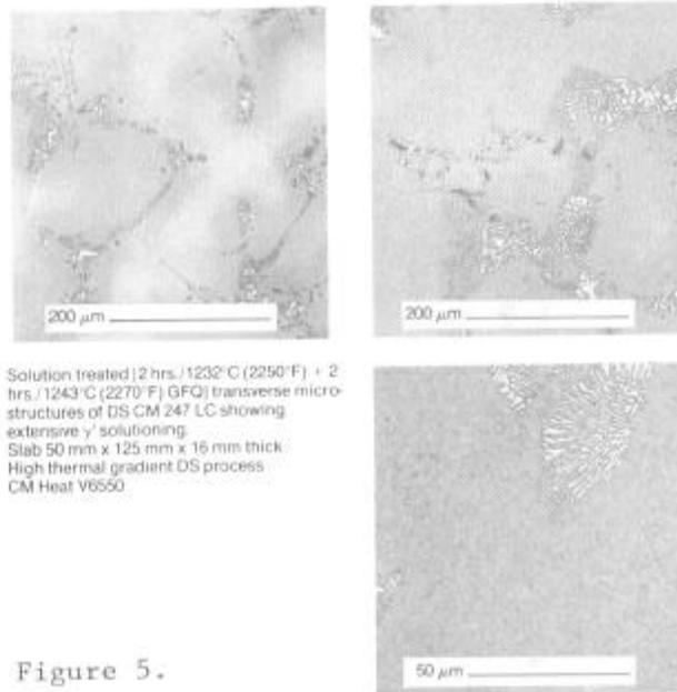
Solution treated (2 hrs./1232°C (2250°F) + 2 hrs./1243°C (2270°F) GFO) transverse microstructures of DS CM 247 LC showing extensive  $\gamma'$  solutioning. Slab 50 mm x 125 mm x 16 mm thick. High thermal gradient DS process. CM Heat V6550.
