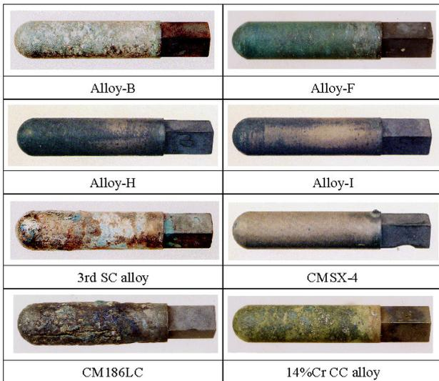
Fig.7. Photos of test specimens after hot corrosion burner rig tests.
