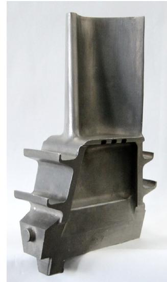
Fig.11. Overview of the single-crystal model bucket (length : 170 mm)
