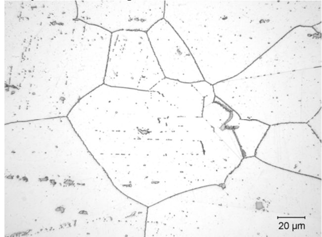
Fig. 2 Age-hardened microstructure of 282 alloy
