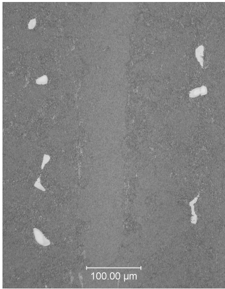
Figure 1. CMSX-7 casting microstructure following solution + double age heat treatment
