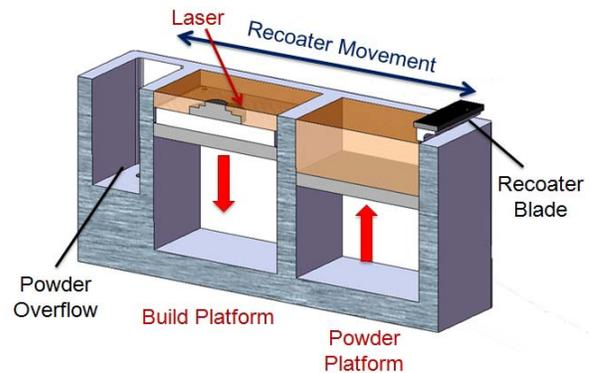
Figure 2. Schematic representation of the Concept Laser M2 Powder Bed Laser Cusing<sup>®</sup> facility. Each subsequent layer of powder is spread over the build area by the movement of the recoater blade and then selectively melted using the computer controlled laser.
