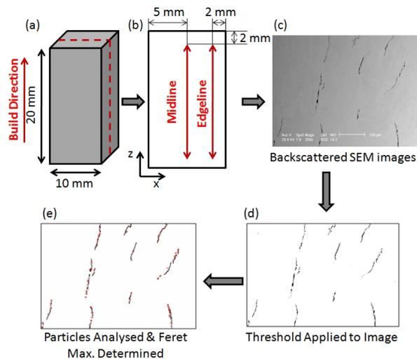
Figure 5. Schematic representation of sampling and analysis method: (a) blocks were sectioned longitudinally (parallel to build direction); (b) 30 images taken along midline and edgeline at 500 $\mu$ m intervals; (c) following standard grinding and polishing, low magnification BSe SEM images reveal cracks; (d) threshold applied to image to isolate cracks; and (e) image analysis carried out to determine feret max. of each crack segment
