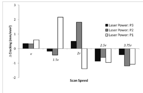
Figure 11. Plot showing  $\Delta$ Cracking (Edgeline Cracking - Midline Cracking values) for complete data sets. The lower energy builds (faster scan speeds) show a clear concentration of the grain-boundary cracking grouped in the middle of the sample.
