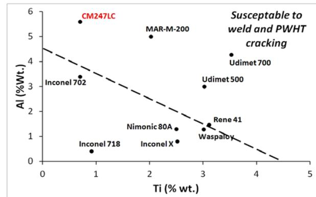
Figure 1. Plot showing increasing cracking susceptibility with  $\gamma'$  forming elements (Al and Ti) [5]. Alloys lying above the dotted line are particularly susceptible to cracking during welding or PWHT.
