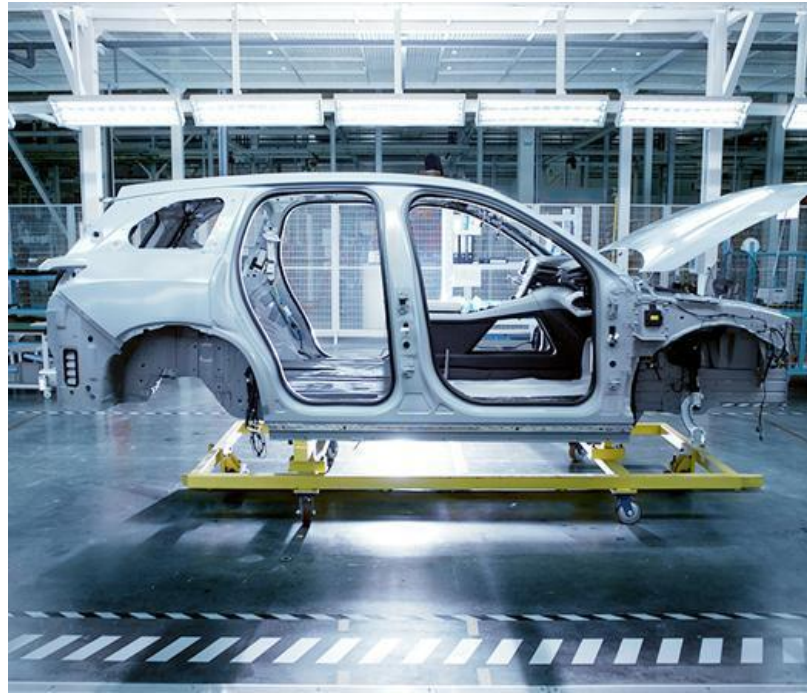
ES8-96.4% is made of aluminium ( 335kg )
