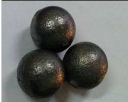
White Iron grinding balls produced from BR iron (21%wt scrap substitution)
